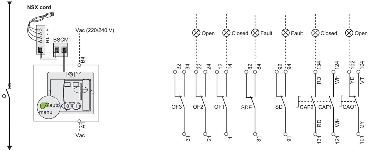
**NOTE:** Schematic of the communicating motor operator .
