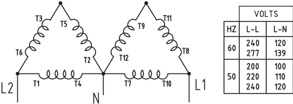
Figure 8-1: 12 Lead Double Delta Single Phase
