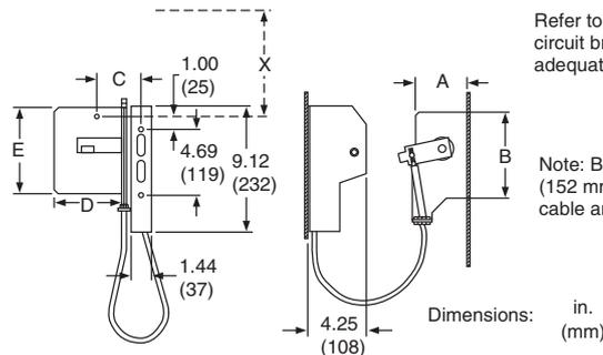
**Table 104: Class 9422 Cable Operating Mechanisms and A1 Handles**
