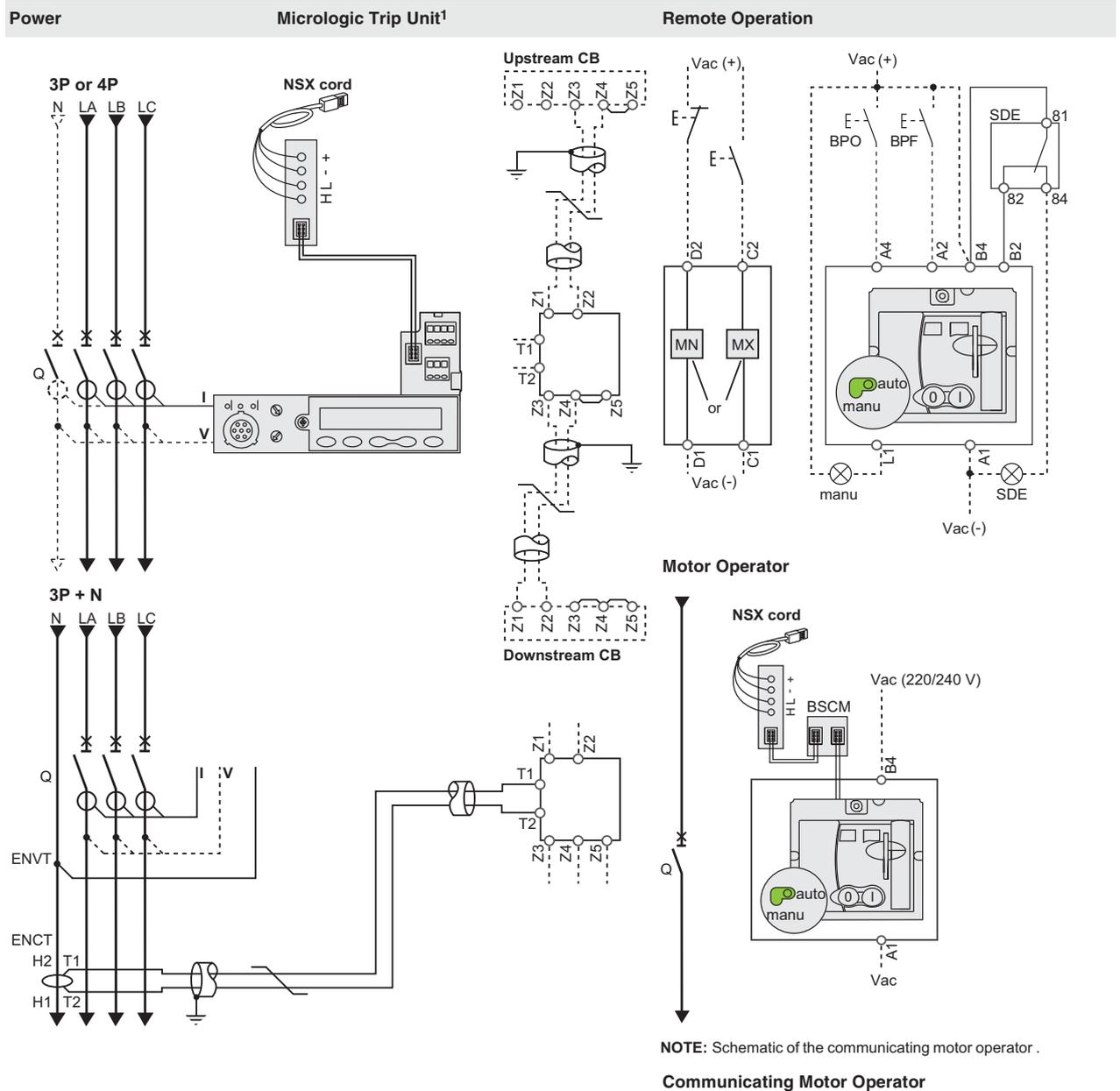
NOTE: Schematic of the communicating motor operator .
