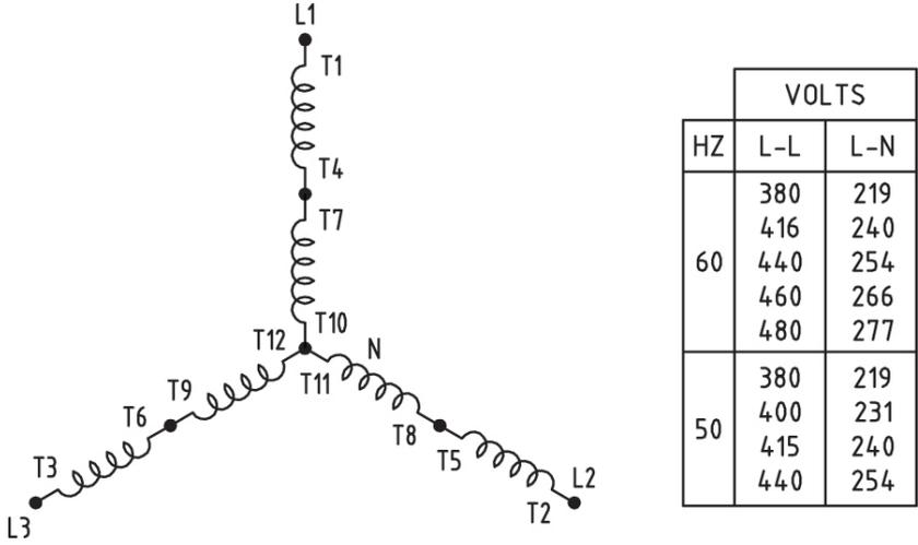
Figure 8-5: 12 Lead Series WYE Three Phase
