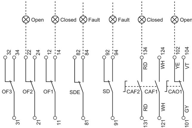
The diagram is shown with circuits de-energized, relays in normal position, and all devices open, connected, and charged. Terminal connections shown as O must be connected by the customer.
