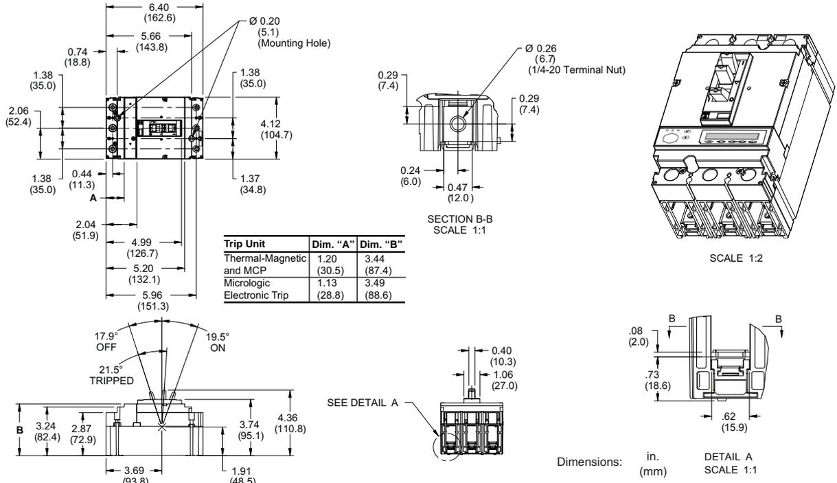
**Figure 16: 15–150 A Lug-Lug PowerPact H-Frame Three-Pole Circuit Breaker**
