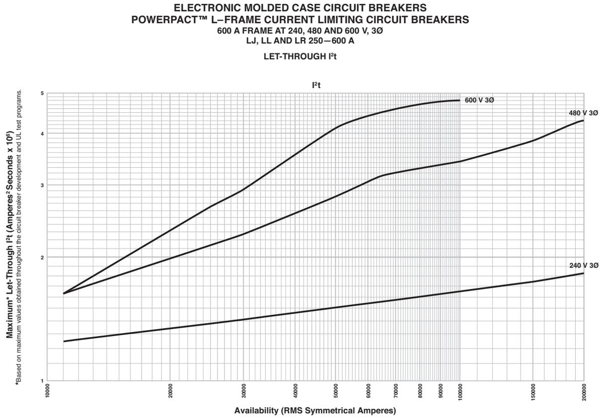
Figure 135: L-Frame Circuit Breaker Reflex Tripping
