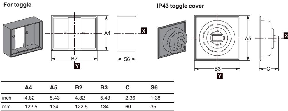
Figure 52: PowerPact L-Frame Circuit Breaker Front-Panel Escutcheons
