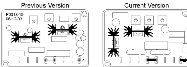
Figure 10. Controller Version Heat Sink Locations
