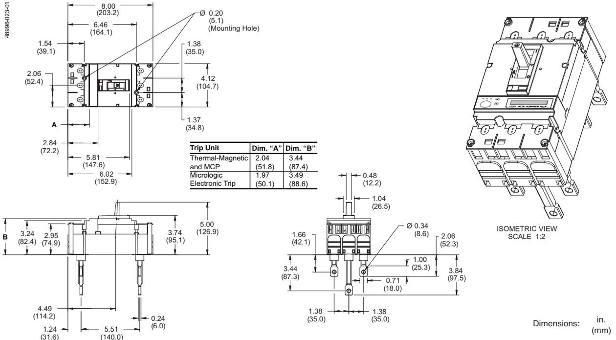
Figure 23: Motor Operator Detail (PowerPact J-Frame Circuit Breaker)
