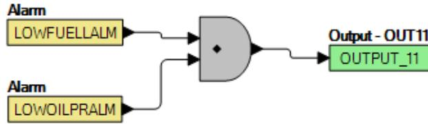
Figure 73. Example 2 – AND Gate Connections
