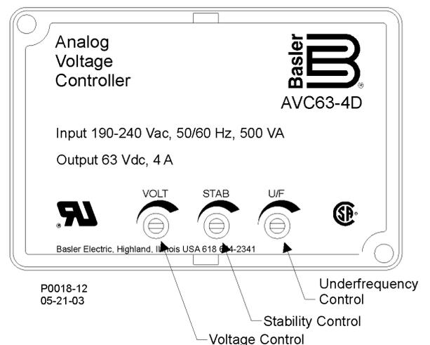
Figure 2. AVC63-4D Potentiometer Control Locations
