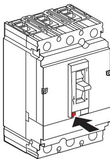
PowerPact H-, J-, and L-frame circuit breakers have an over-center toggle mechanism providing quick-make, quick-break operation. The operating mechanism is also trip-free, which allows tripping even when the circuit breaker handle is held in the “ON” position.
