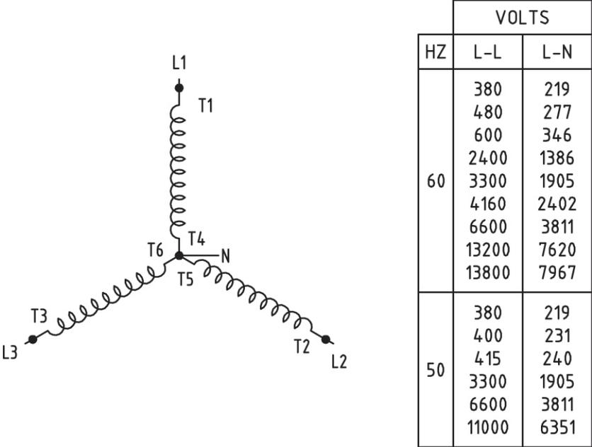
Figure 8-7: 6 Lead WYE Three Phase
