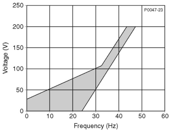
Figure 5. Frequency Compensation Characteristic - 50 Hz
