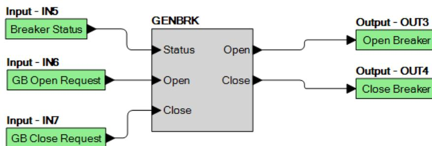
Figure 72. Example 1 – GENBRK Logic Block Connections
