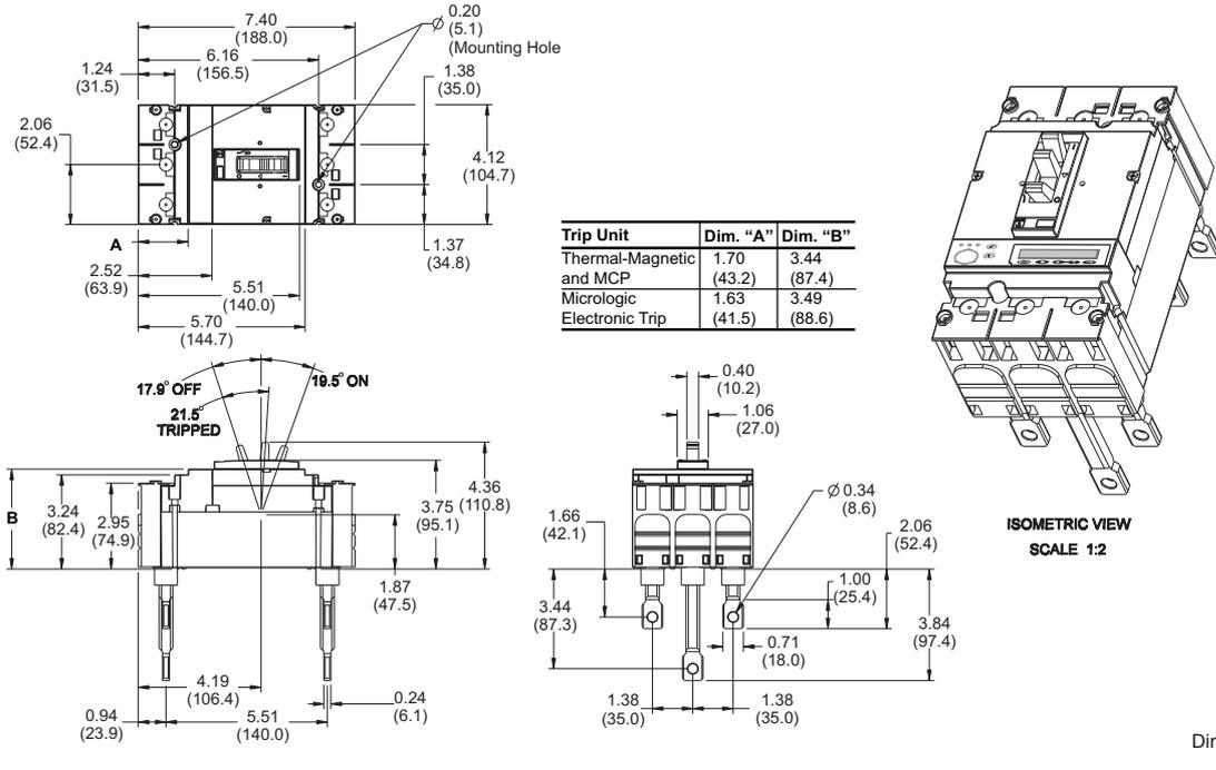
Figure 18: Motor Operator Detail (PowerPact H-Frame Circuit Breaker)
