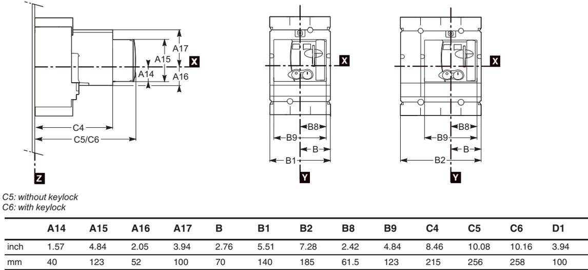
**Figure 46: PowerPact L-Frame Circuit Breaker Motor Operator Front-Panel Cutouts**
