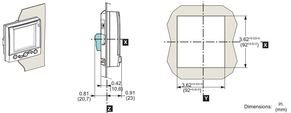
**Figure 66: FDM121 Switchboard Display Mounting On Panel**
