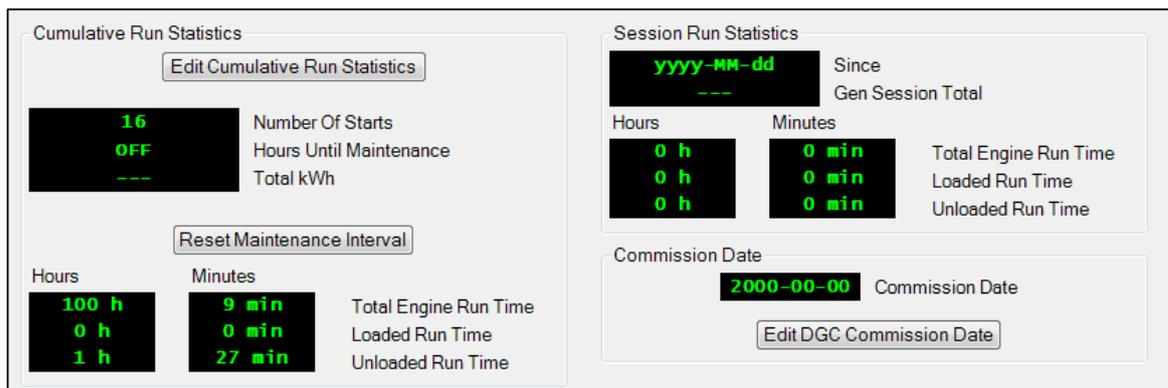
Figure 30. Metering Explorer, Run Statistics Screen
