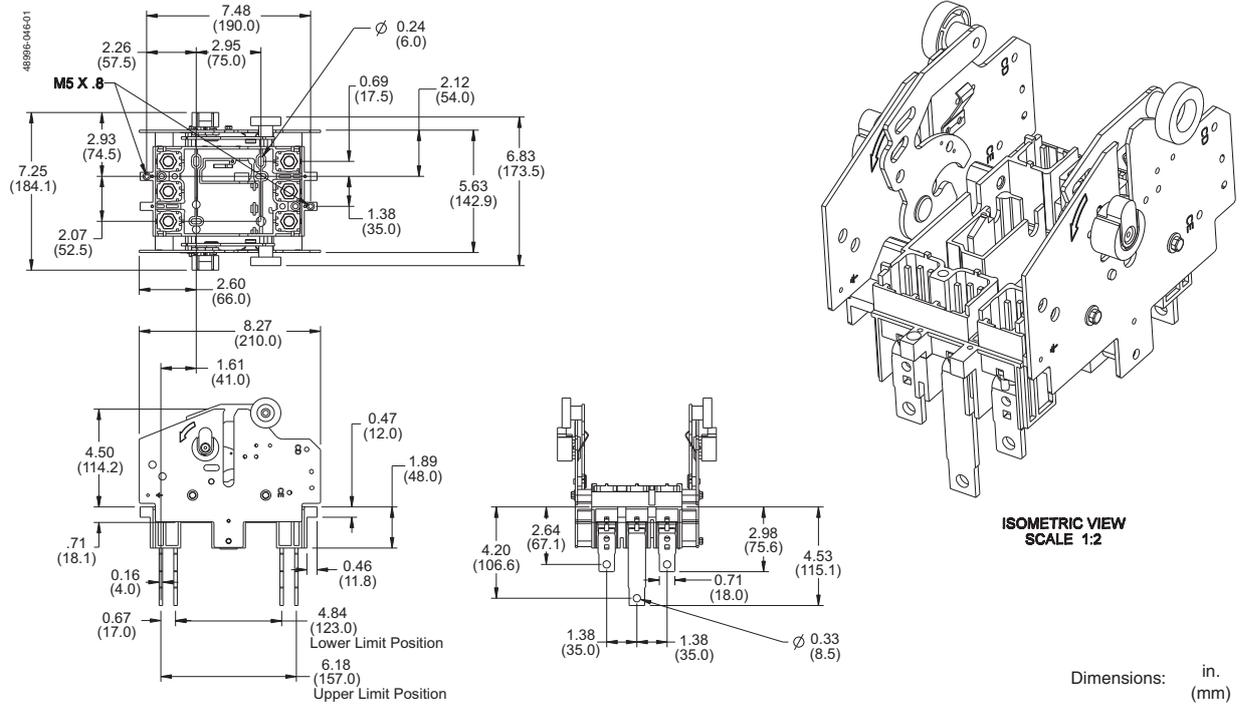
Figure 28: 15–250 A PowerPact H- and J-Frame Drawout Three-Pole Circuit Breaker
