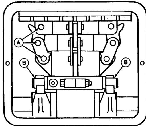
Lubrication Internal Parts of PTO Clutch
