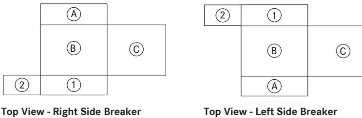
**Figure 2: 280 Frame Enclosure Breaker Mounting Positions**
