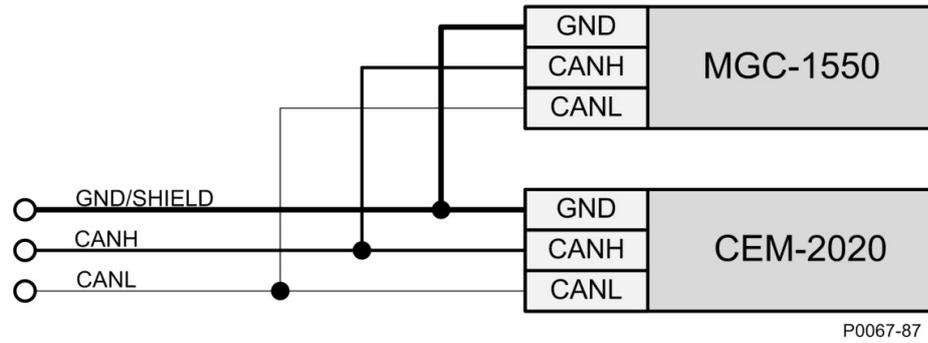
Figure 55. MGC-1550 and CEM-2020 CAN Connections
