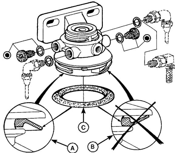
Fuel Filter Dust Seal Installation
