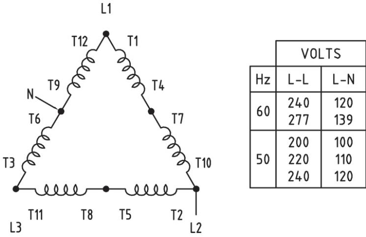
Figure 8-4: 12 Lead Series Delta Three Phase
