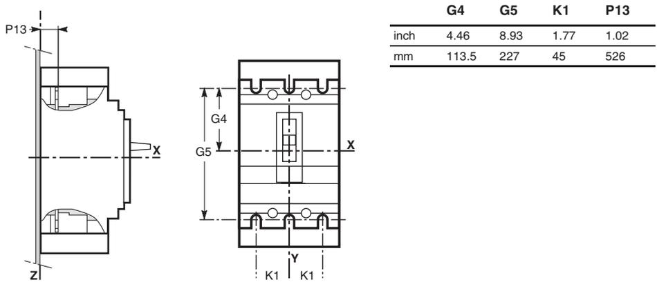
Figure 56: PowerPact L-Frame Circuit Breaker Front Connections
