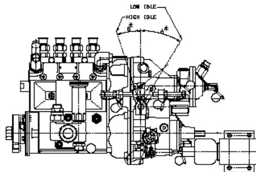
Figure 12-3: Standard Mechanical Governor for Diesel Engines
