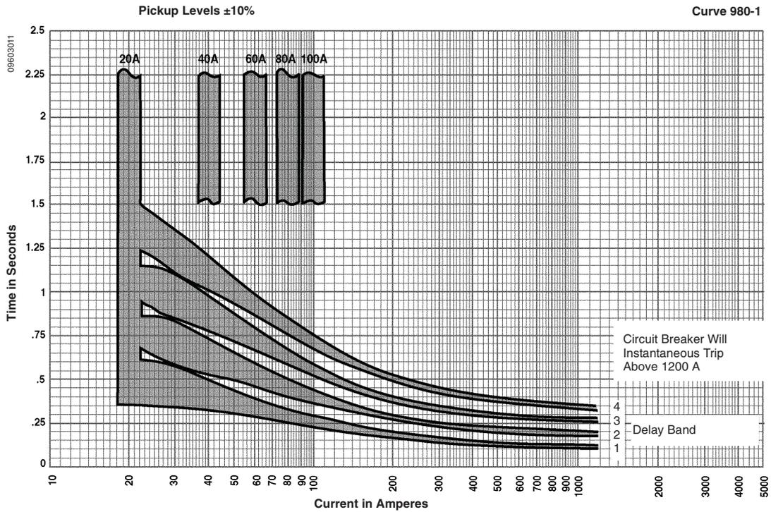
Figure 99: Ground Fault Module GFM250JD Trip Curve
