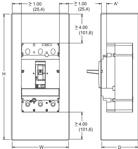
If dimension A < 0.56 in. for H- and J-frame circuit breaker, attach fiber insulating plate, not provided, to enclosure cover.
