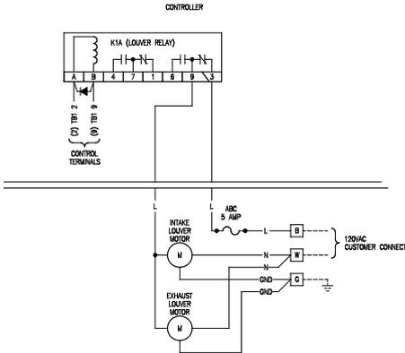
Figure 8-9: Optional motorized louver wiring
