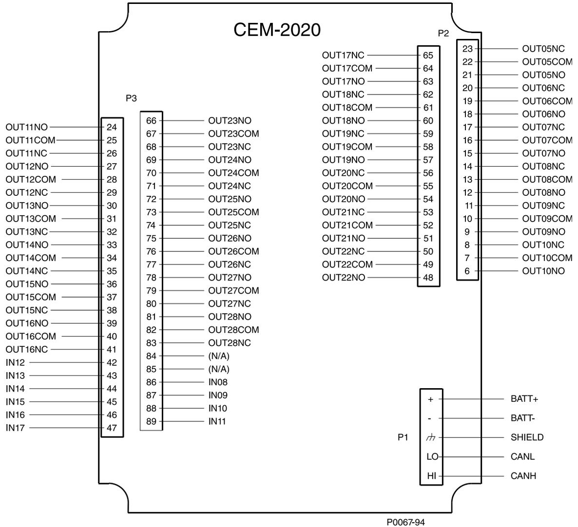
Figure 93. CEM-200 Contact Input and Contact Output Terminals
