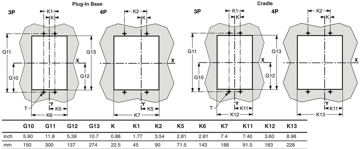
Figure 43: PowerPact L-Frame Circuit Breaker Mounting on Rails (Plug-In Base or Cradle)
