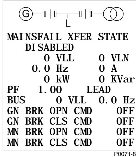
Figure 5. One-Line Diagram Menu Options (Available when One-Line Diagram is Enabled)
