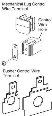
Powerpact H- and J-Frame mechanical lugs may be equipped with a separate control wire termination. The kit is available factory installed or as a field installable kit. The adaptor is secured underneath the lug and has a tab extension suitable for attachment of a 0.250 inch slip-on connector.
