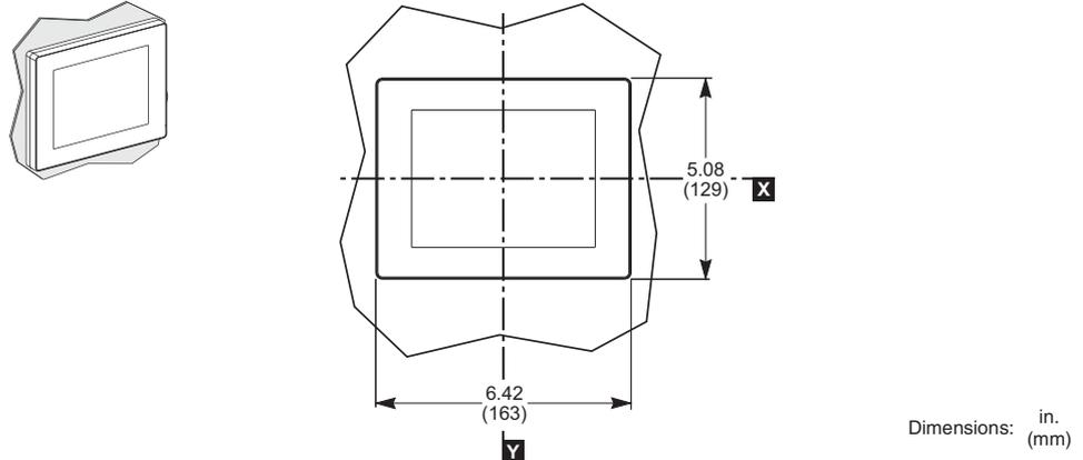
Figure 68: FDM128 Switchboard Display Mounting on Panel
