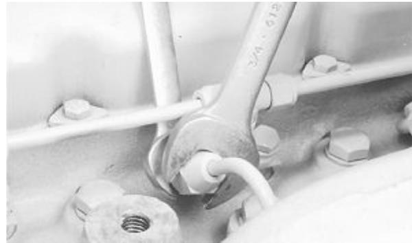
Bleeding Fuel System at Injection Nozzle
