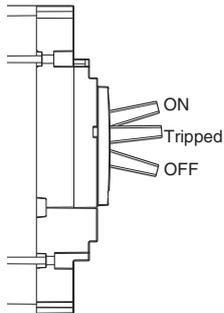
The circuit breaker handle can assume any of three positions, ON, tripped or OFF as shown. The center tripped position provides positive visual indication that the circuit breaker has tripped.
