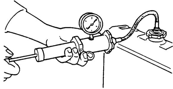
Pressure Testing Cooling System
