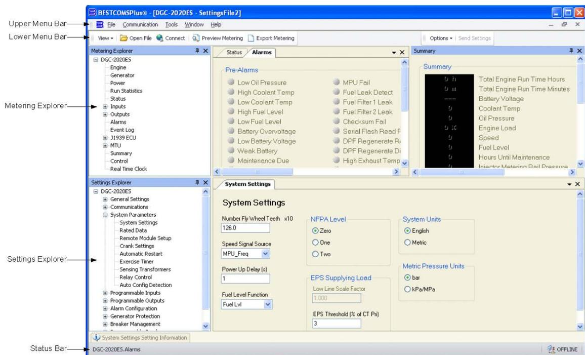
Figure 56. Typical User Interface Components
