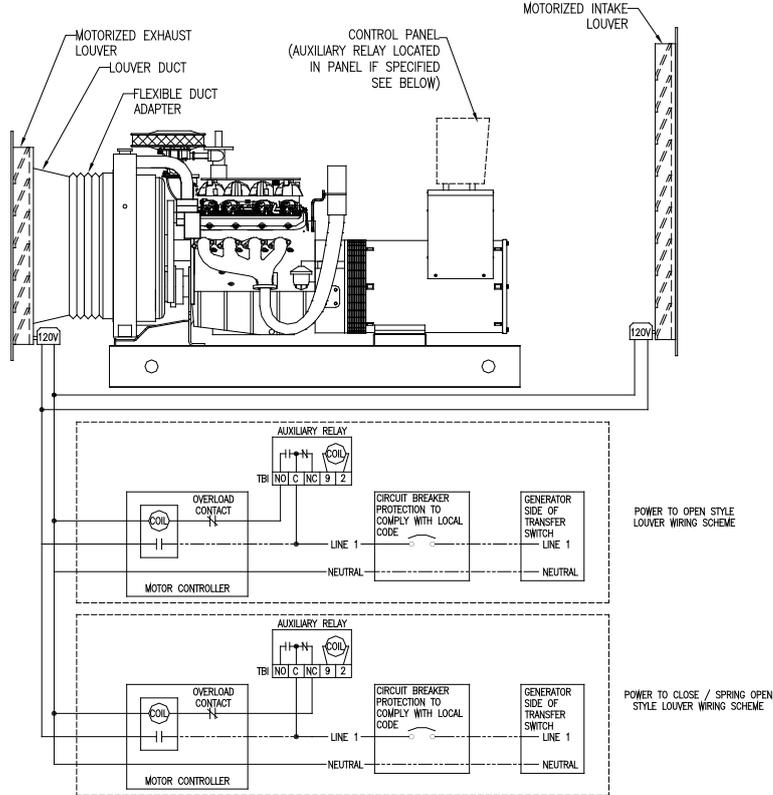
Figure 8-8: Suggested motorized louver wiring
