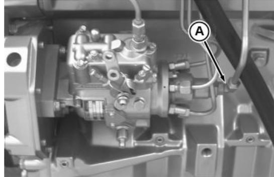
Fuel Supply Line Connector at Injection Pump
