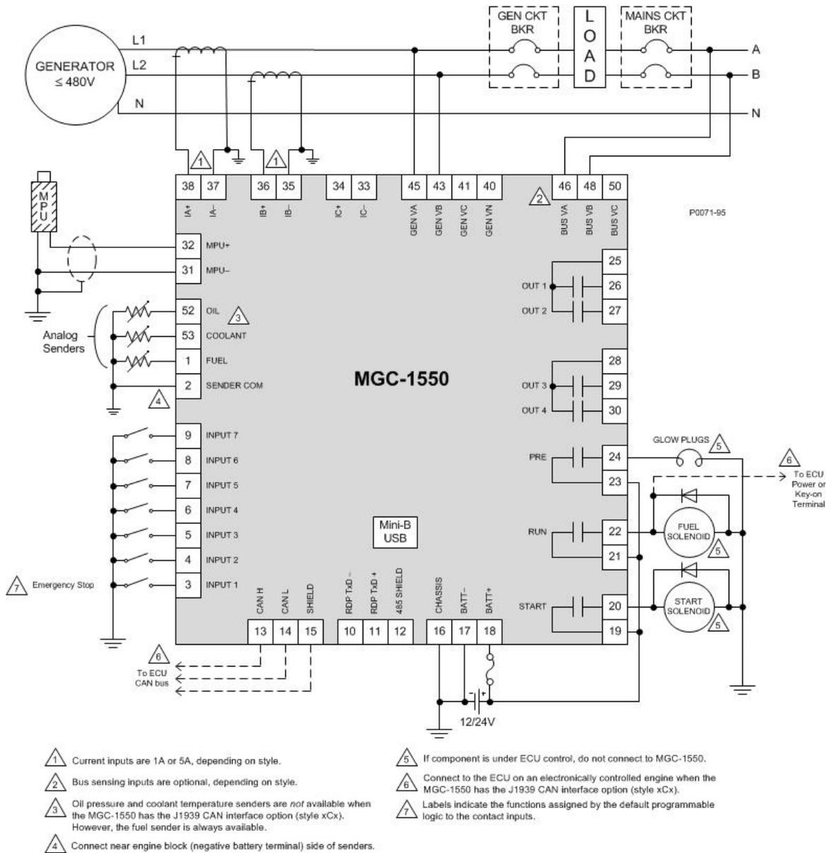
Figure 51. Single-Phase A-B Connections for Typical Applications
