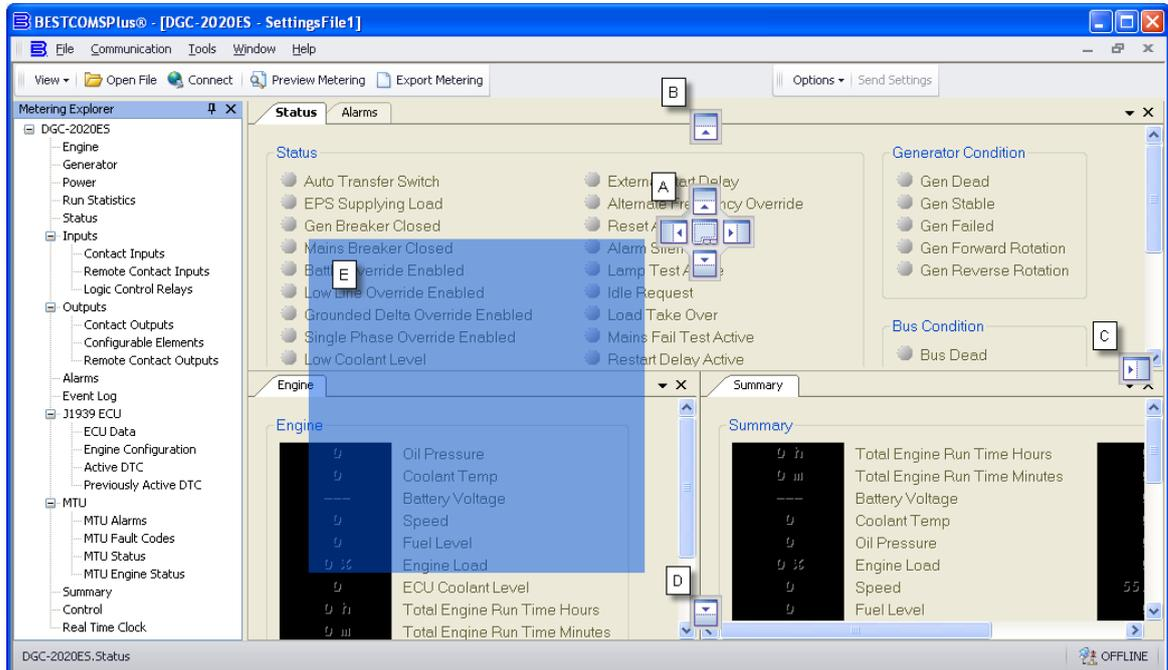
Figure 26. Metering Screen Docking Options
