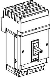
I-Line circuit breakers use “blow-on” type line side connectors. In case of a short circuit, increased magnetic flux causes the plug-on connectors of the circuit breaker to tighten their grasp on the bus bars. The I-Line connectors and circuit breaker mounting bracket are integral parts of I-Line circuit breakers and cannot be removed or replaced. I-Line circuit breakers come with mechanical load side lugs, or optional terminal nut to connect to bus bars or to compression (crimp) lugs.
