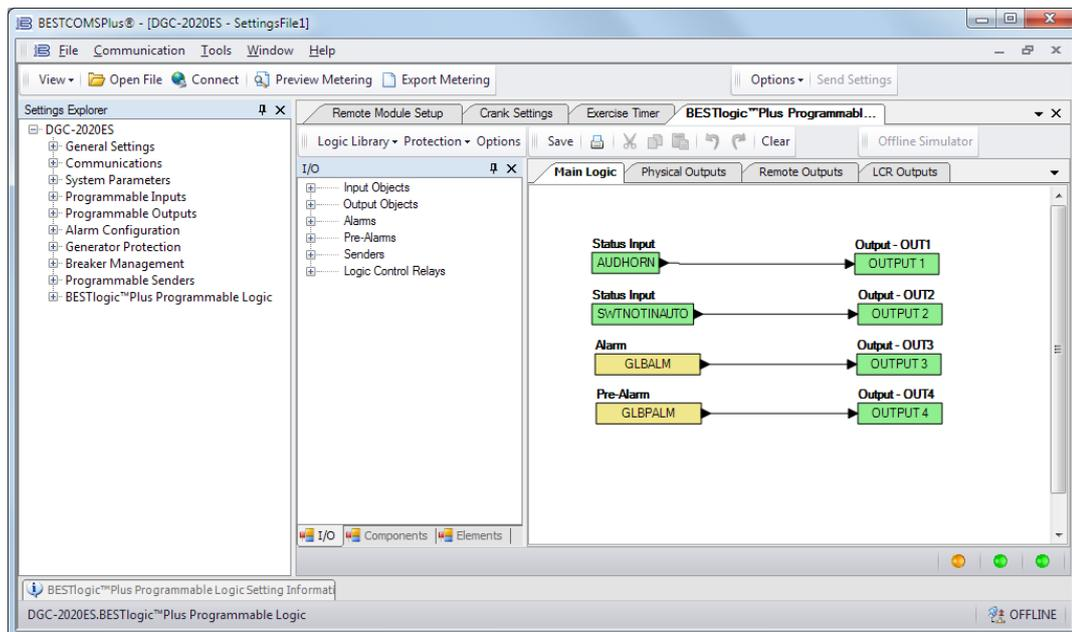
Figure 68. Settings Explorer, BESTlogicPlus Programmable Logic Screen
