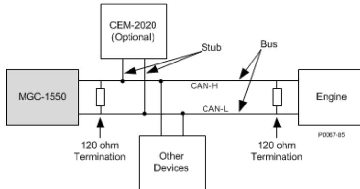
Figure 95. CAN Interface with MGC-1550 providing One End of the Bus
