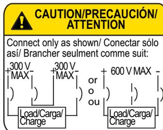
L-Frame Three-Pole Circuit Breakers
