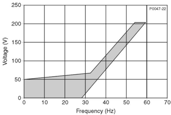
Figure 4. Frequency Compensation Characteristic - 60 Hz
