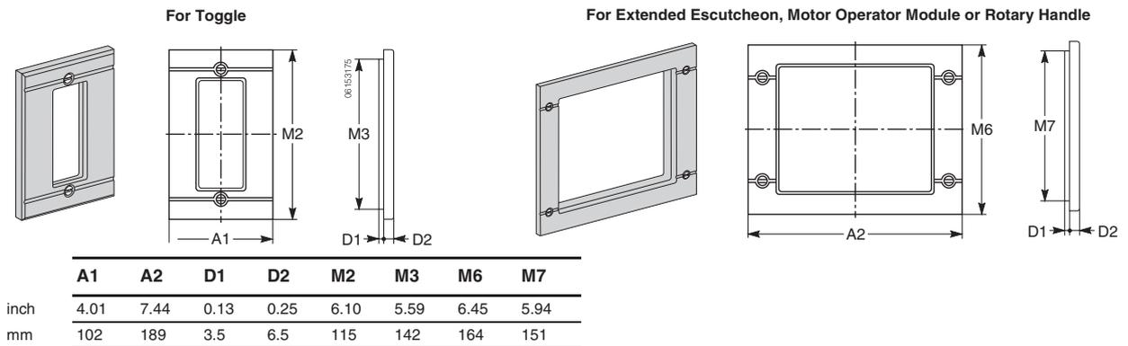
**PowerPact H-, J-, and L-Frame Circuit Breakers
