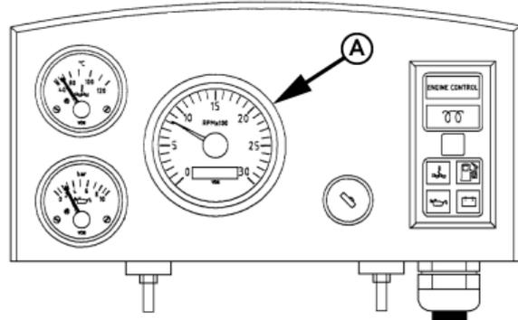
VDO Instrument Panel Tachometer
