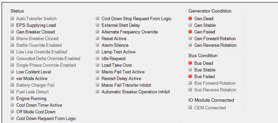
Figure 31. Metering Explorer, Status Screen
