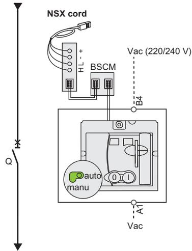
**NOTE:** Schematic of the communicating motor operator .
