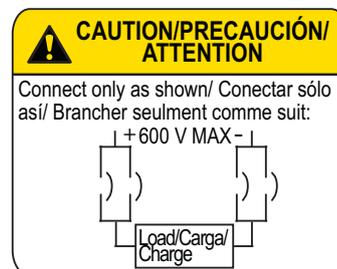
L-Frame Four-Pole Circuit Breakers
