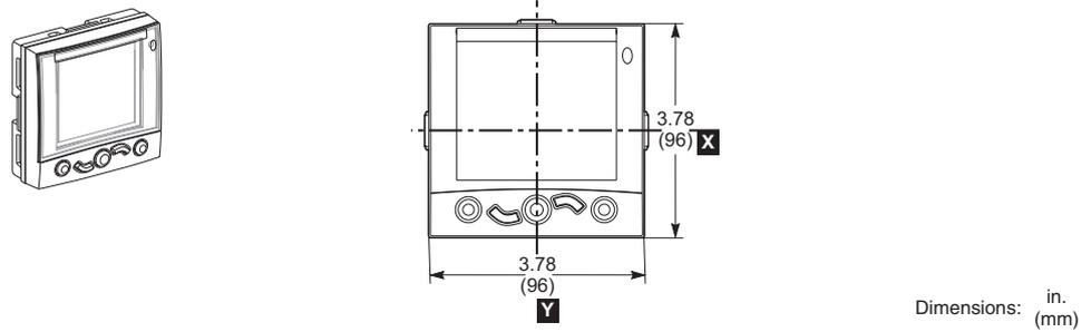
**Figure 65: FDM121 Switchboard Display Mounting Through Panel**
