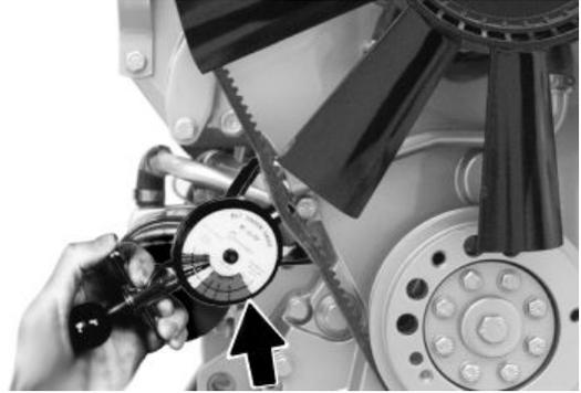
Checking Belt Tension with Tension Gauge
