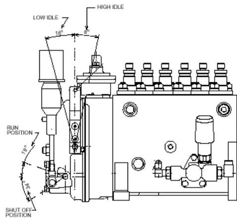
Figure 12-2: Standard Mechanical Governor for Diesel Engines
