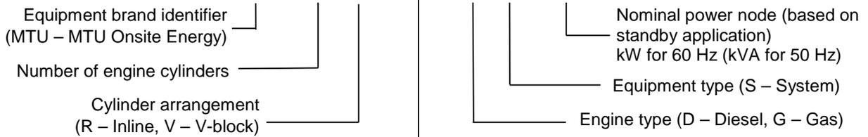
MTU Series or nominal displacement per cylinder (4-digit identifier)
