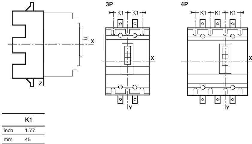
**Figure 59: PowerPact L-Frame Circuit Breaker Rear Connections Fitted at Lower Limit**
