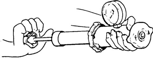
Pressure Testing Radiator Cap
