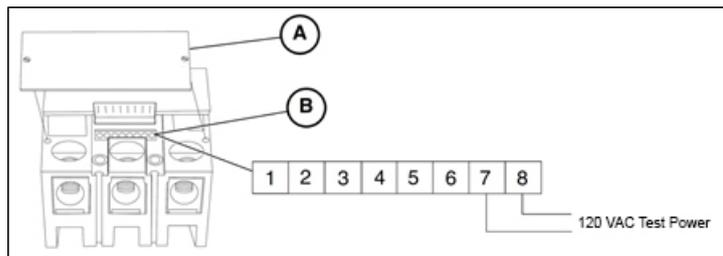
**Figure 1: Lug cover for access to terminals 7 and 8**
