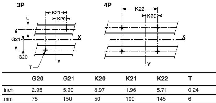
Figure 44: PowerPact L-Frame Circuit Breaker Front-Panel Cutouts
