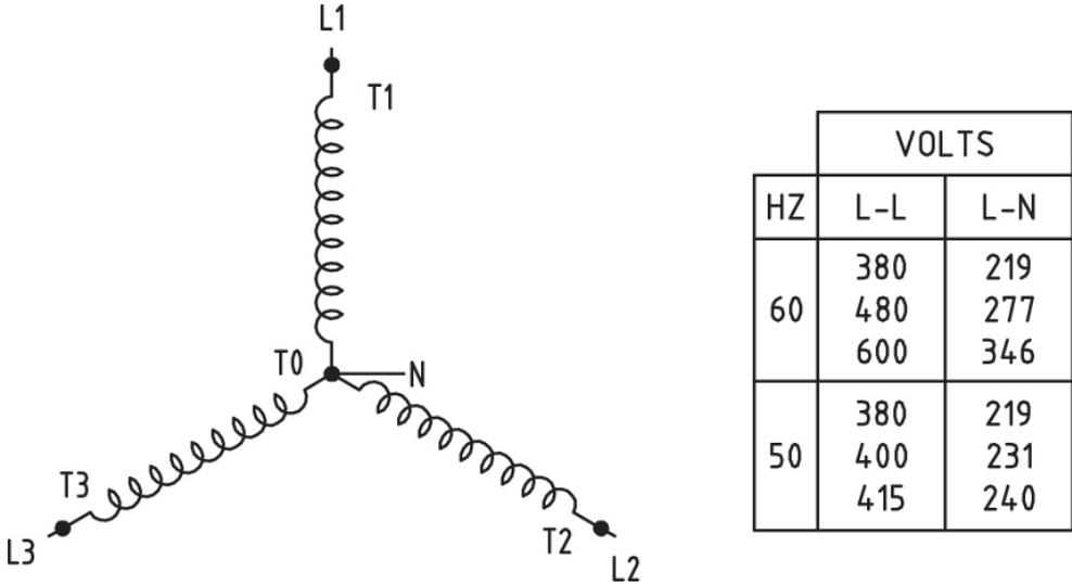
Figure 8-6: 4 Lead WYE Three Phase
