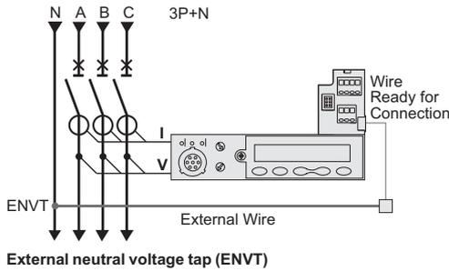
This connection is required for accurate power measurements on three-pole circuit breakers equipped with Micrologic 5/6 E trip units in installations with a distributed neutral. It can be used to measure phase-neutral voltages and calculate power using the 3 wattmeter method.
