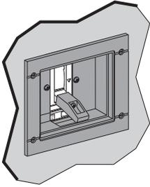
Toggle collars make it possible to maintain degrees of protection regardless of the circuit breaker position (connected, disconnected):
