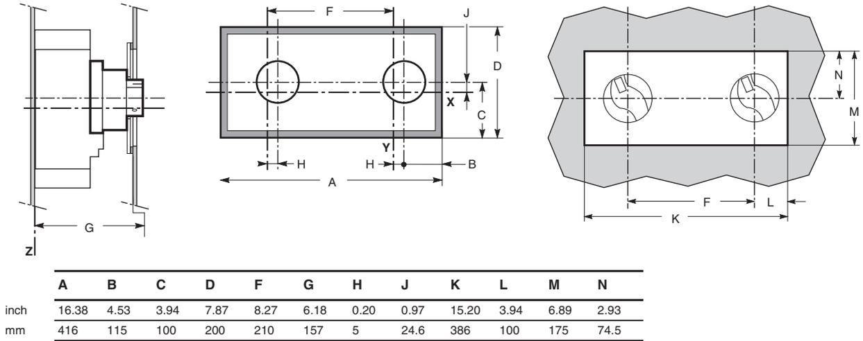
**Figure 54: PowerPact L-Frame Circuit Breaker Interlocking Systems with Toggle Handles**
