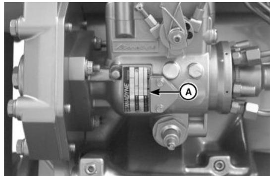
*Injection Pump Serial Number Plate*
