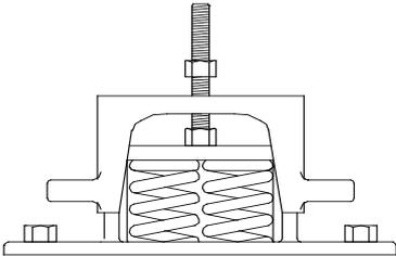
Figure 4-2: Spring mount vibration isolator
