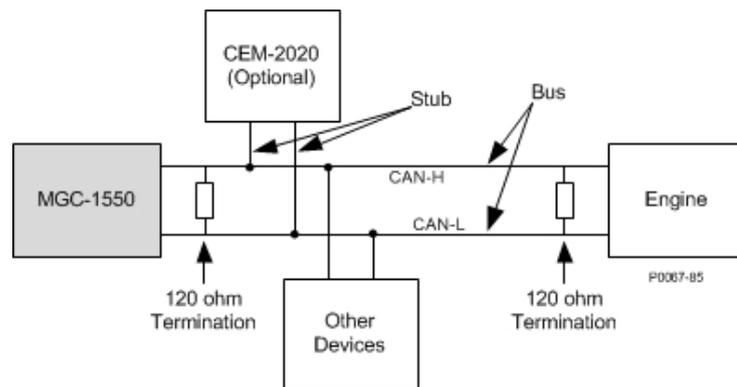
Figure 53. CAN Interface with MGC-1550 Providing One End of the Bus
