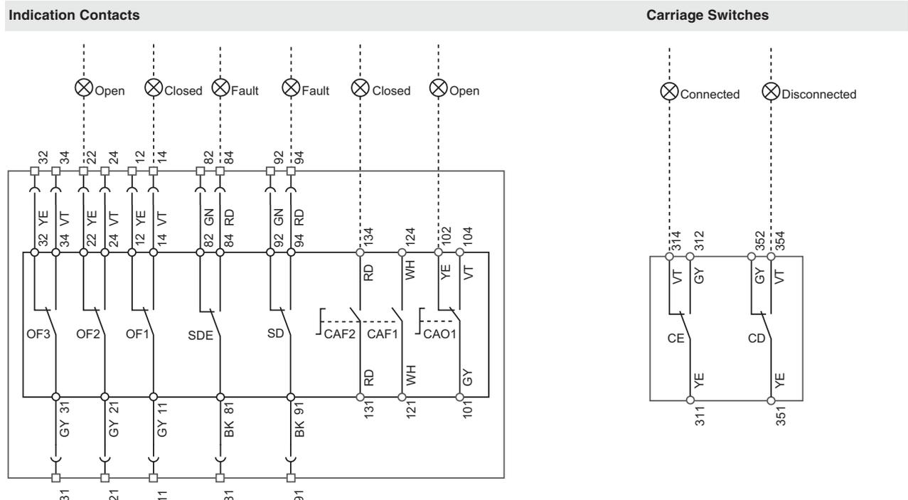
The diagram is shown with circuits de-energized, relays in normal position, and all devices open, connected, and charged. Terminal connections shown as □ and ○ must be connected by the customer.
