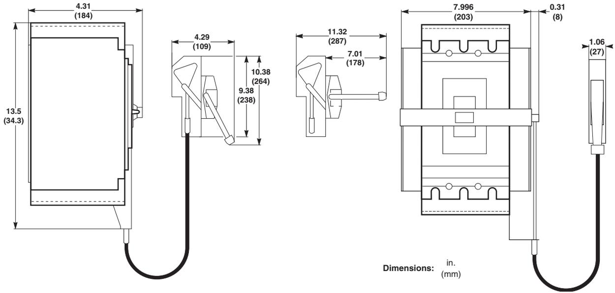
Figure 48: PowerPact L-Frame Circuit Breaker Rotary-Operating Handles
