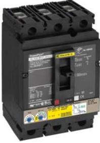
PowerPact H- and J-frame Electronic Motor Circuit Protectors (MCP) are instantaneous-trip circuit breakers. They are designed to offer short circuit protection and are National Electrical Code® (NEC®) compliant when installed as part of a combination controller having motor overload protection. MCP circuit breakers accept the same accessories and terminals as the equivalent thermal-magnetic circuit breakers. (See Section 3 for Accessories.)
