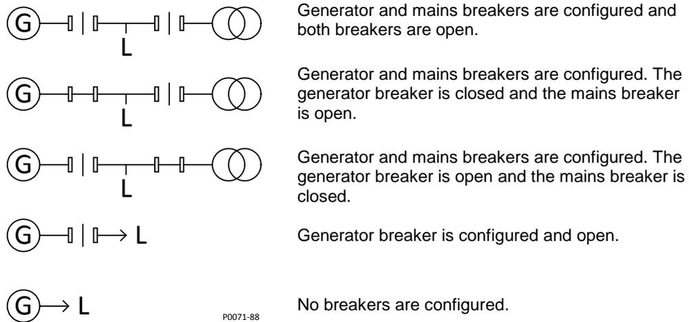
Figure 6. One-Line Diagram: Breaker Hardware Status Indication
