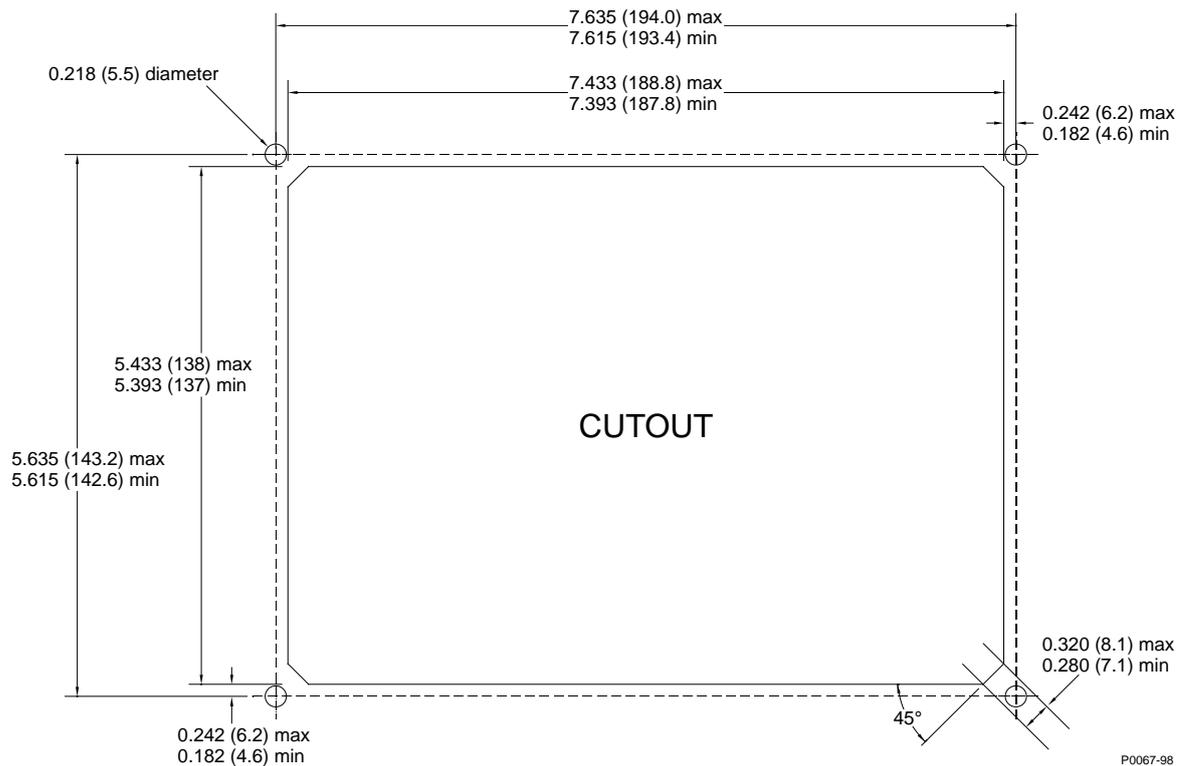
Figure 46. Panel Cutting and Drilling Dimensions
