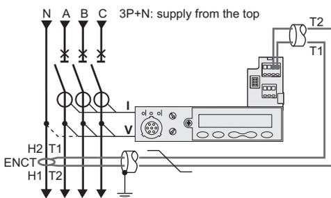
This connection is required to protect the neutral on three-pole circuit breakers equipped with Micrologic 5/6 A or E trip units in installations with a distributed neutral. For Micrologic 6 A or E, it is required for ground-fault protection.
