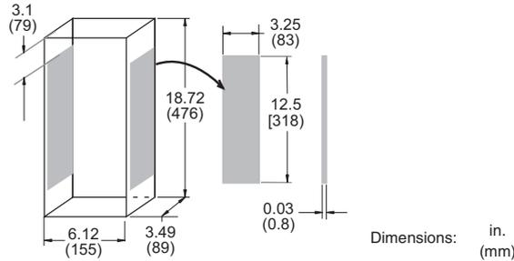
**L-Frame Minimum Enclosure Insulation for Rear Connection**
