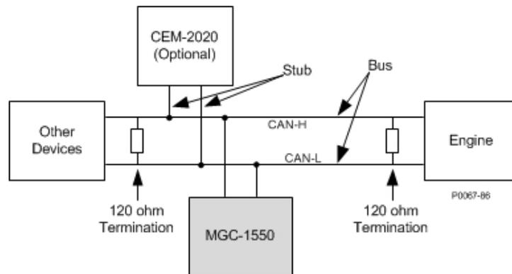
Figure 54. CAN Interface with Other Devices
