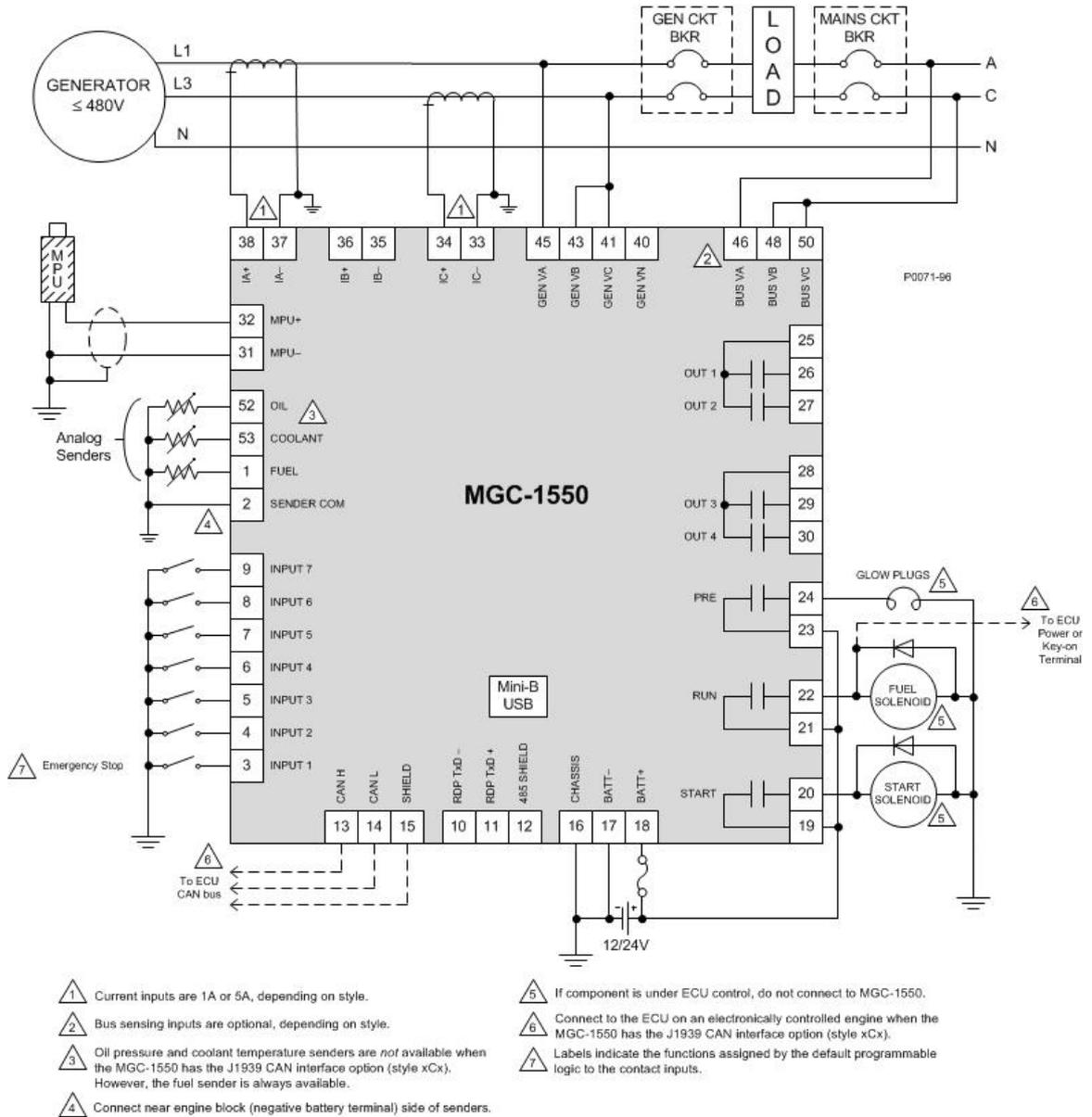
Figure 52. Single-Phase A-C Connections for Typical Applications
