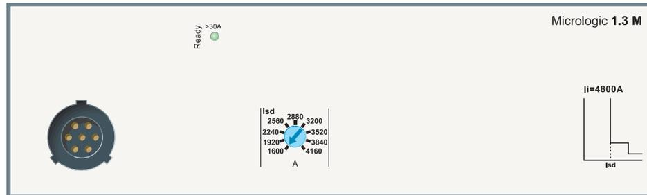
Micrologic 1.3 M trip units provide instantaneous protection only, using electronic technology. They are dedicated to 600 A three-pole (3P 3D) circuit breakers or four-pole circuit breakers with detection on three poles (4P, 3D). They are especially used in three-pole versions for motor protection.
