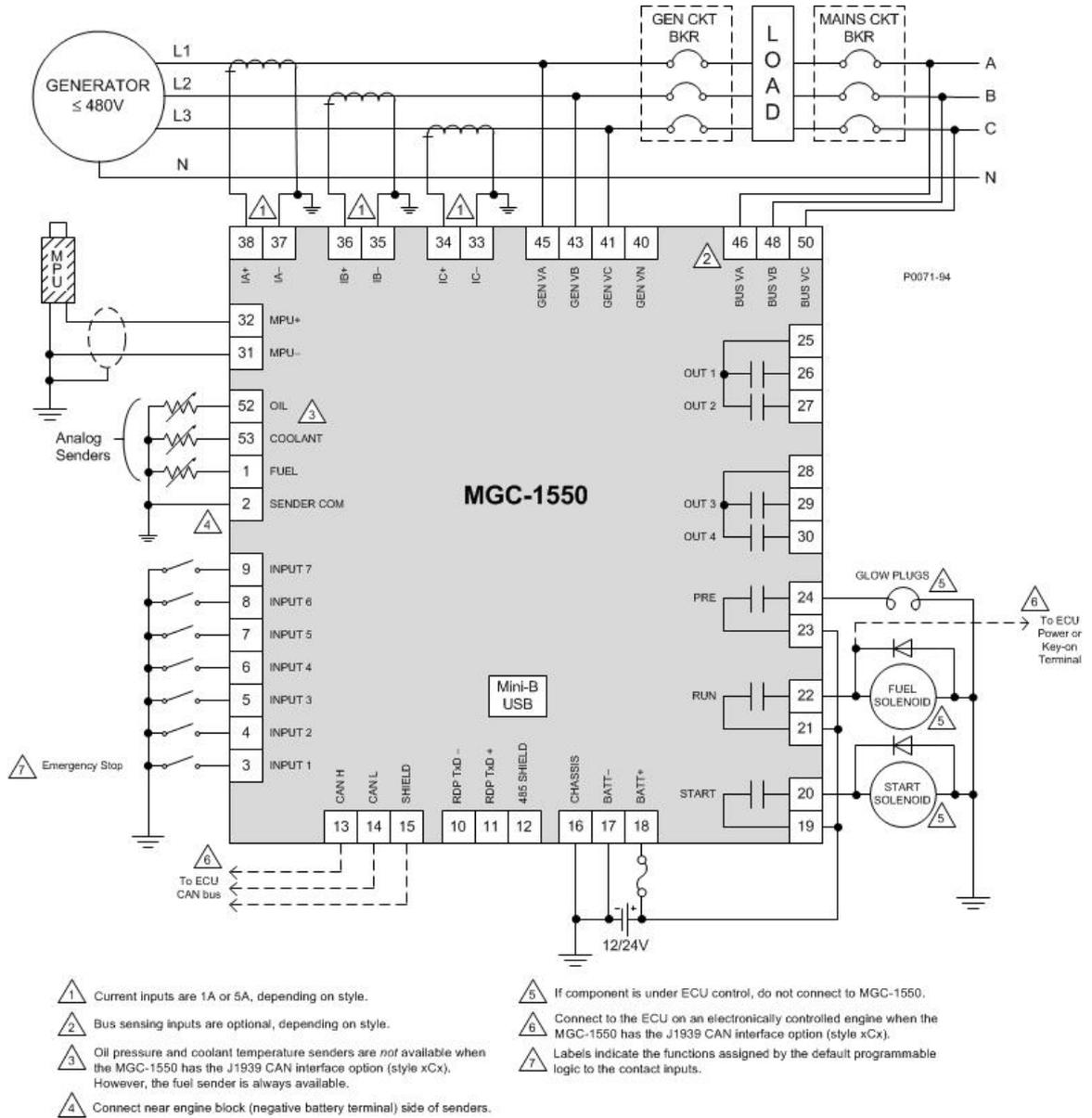
Figure 50. 3-Phase Delta Connections for Typical Applications
