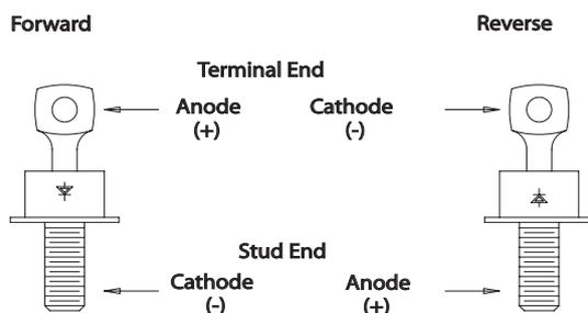
FIGURE 4: DIODE POLARITY
