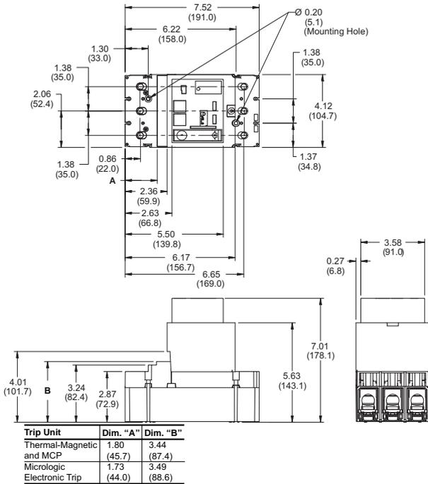
Figure 24: Rotary Handle Detail (PowerPact J-Frame Circuit Breaker)
