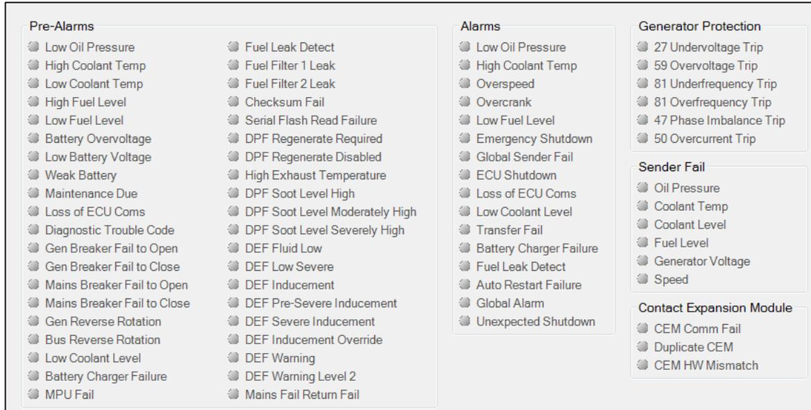
Figure 44. Metering Explorer, Alarms Screen
